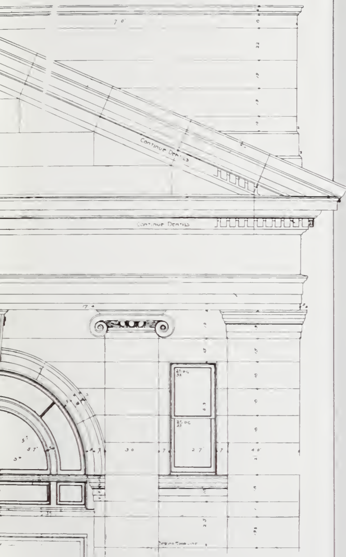
HALF-ELEVATION ABOVE SECOND FLOOR REAR CENTER WING
